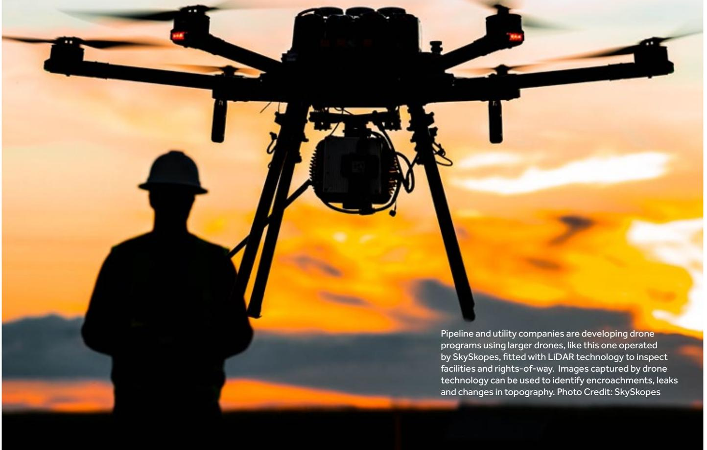
Pipeline and utility companies are developing drone programs using larger drones, like this one operated by SkySkopes, fitted with LiDAR technology to inspect facilities and rights-of-way. Images captured by drone technology can be used to identify encroachments, leaks and changes in topography. Photo Credit: SkySkopes
