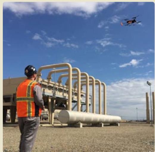
A Pacific Gas and Electric Company technician tests a methane gas sensor attached to a small drone. Photo Credit: Pacific Gas and Electric Company
